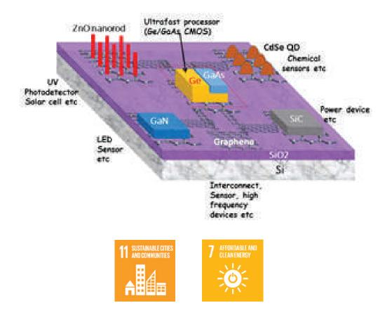
Micro-nanodevice Area : Novel nanodevices and functional devices covering electronic/photonic devices, microfluidic devices, sensors and solar cells. Three-branch junction device Micromixer DNA Sensors
