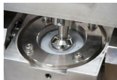
Fig.2 Hip joint model installed in hip joint simulator
